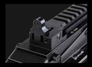
PZD 556 MK2 has adjustable diopter rear sights to improve the speed of target acquisition.
