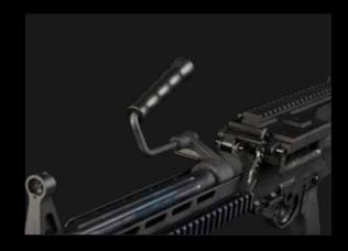
PZD 762 Mk1 uses a quick change flueted barrels that improve the heat dissipation allowing the operator to sustain the operation of the machine gun for longer period of time without changing the barrel. Barrel comes with adjustable front sight and are zeroed identically to ensure there is no change in ballistics when swapped.
