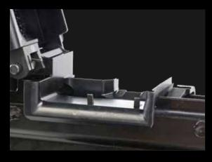
Modified feed tray with two retaining paws that hold the belt on the feed tray under any circumstances. This feature adds significant improvement when reloading or operating with NVGs.
